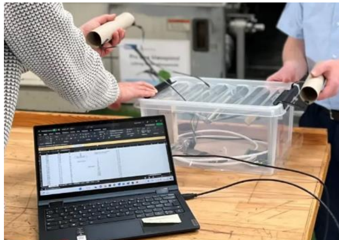
Figure 4. Initial tests of strain gauges in controlled environment.
