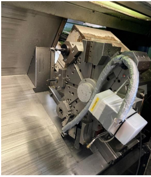
Figure 13. Cable routing and machine crash during revolver rotation.
