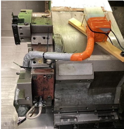
Figure 22. New mount with better waterproof electronics box
