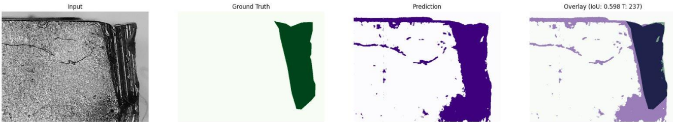
Figure 17 Sample from training process, from left: input source image, annotated mask, prediction by the model and overlay of annotated and predicted mask.
