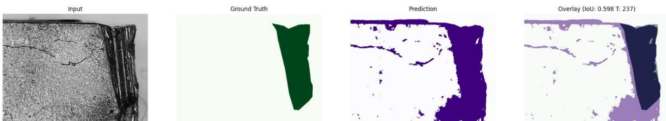
Figure 31 Sample from training process, from left: the input image, annotated mask, prediction from the model and rightmost overlay of annotated mask and predicted mask.
