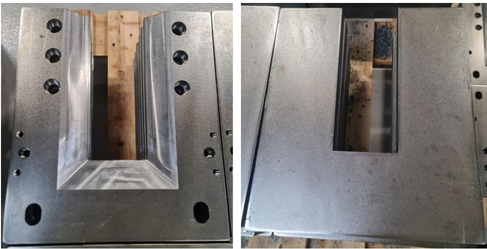
Figure 44 – Final machined part (left) and rough material (right).
