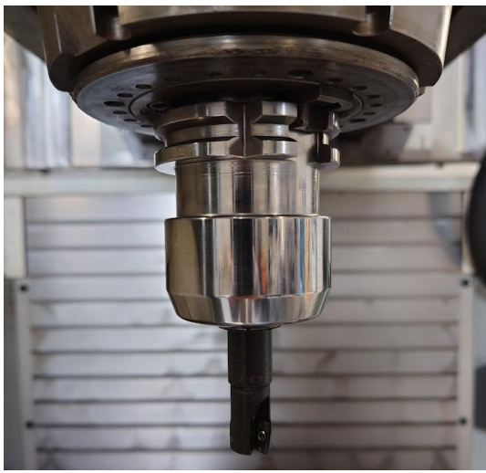
Figure 27 – The tool used during the tests of the boring cutting module.
