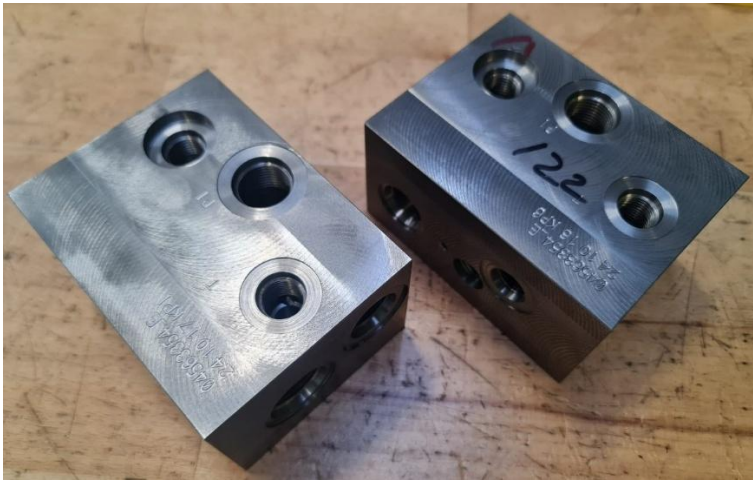
Figure 48 – Machined parts, optimized parameters (left) and base case part (right).
