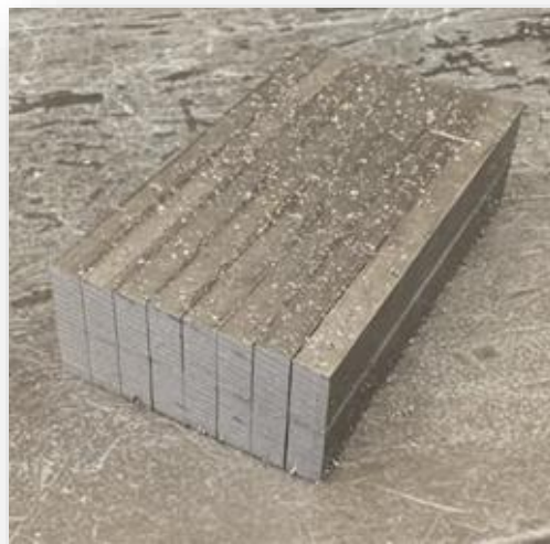
Figure 22: Sixteen sections of flat bar stacked together via welding
